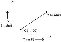
Above graph represents a reversible process  $X \to Y$  of one mole of an ideal gas. The values of pressure and temperature of the systems X and Y are mentioned in the brackets.
